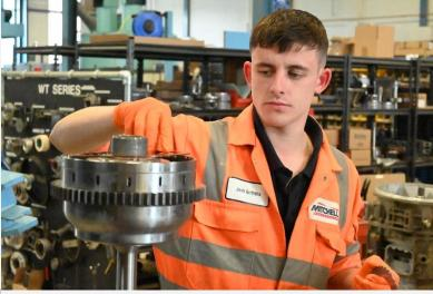
Every transmission is overhauled from the ground up. Transmissions are disassembled part-by-part to clean, qualify and test. Each component is screened for the possibility of reuse to minimise cost for the customer.
