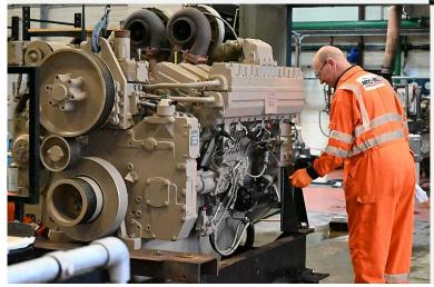
Our engine test cell can handle most brands of diesel engines up to 3000bhp, and we can facilitate complete engine dynamometer testing to verify performance under expected operating conditions. FAT's can also be facilitated (optional upon request).
